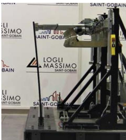
Test a carico statico SLU, 3,0 kN/m, Hs=120 cm
