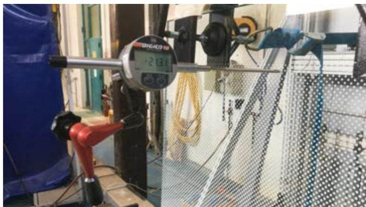
Test a carico statico SLE, 1.0 kN/m, Hspinta= 110 cm
