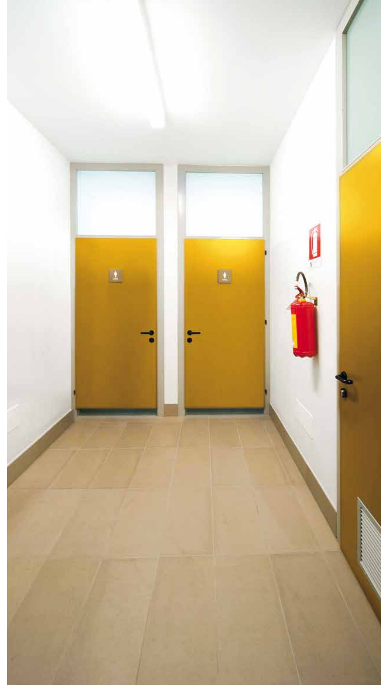
plastic collection Art. 11P porta a battente con sopraluce hinged door with upper window laminato - laminate finishing SP. TH. 9/10 vetro trasparente - transparent glass Mod. 01A cassa in pvc - pvc doorframe Mod. telescopic PP41B
